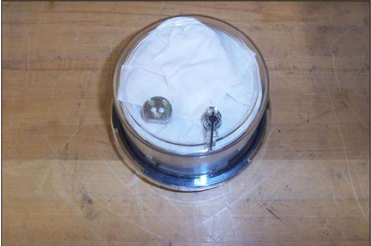
**Photograph 74. Test No. 38: Rain-Tightness, Meter Serial No. 10298, After – 2**
