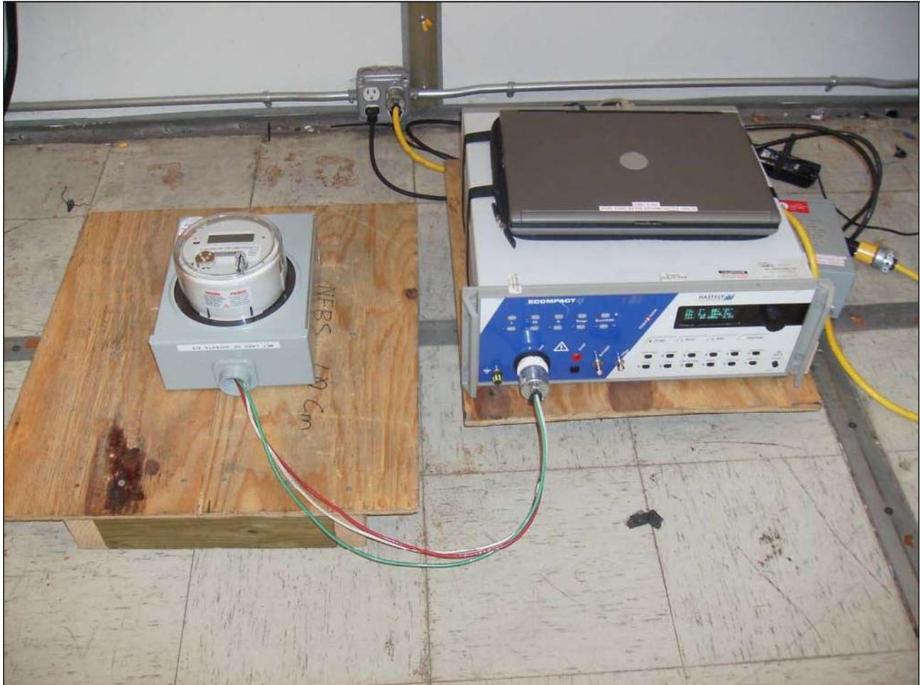
Photograph 17. Test No. 16: Voltage Interruptions Test, Test Setup
