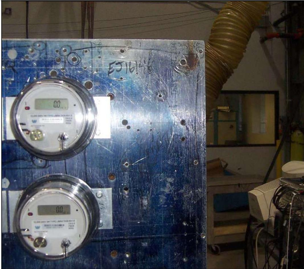
Photograph 40. Test No. 32: Mechanical Shock, X-Axis, Test Setup – 2
