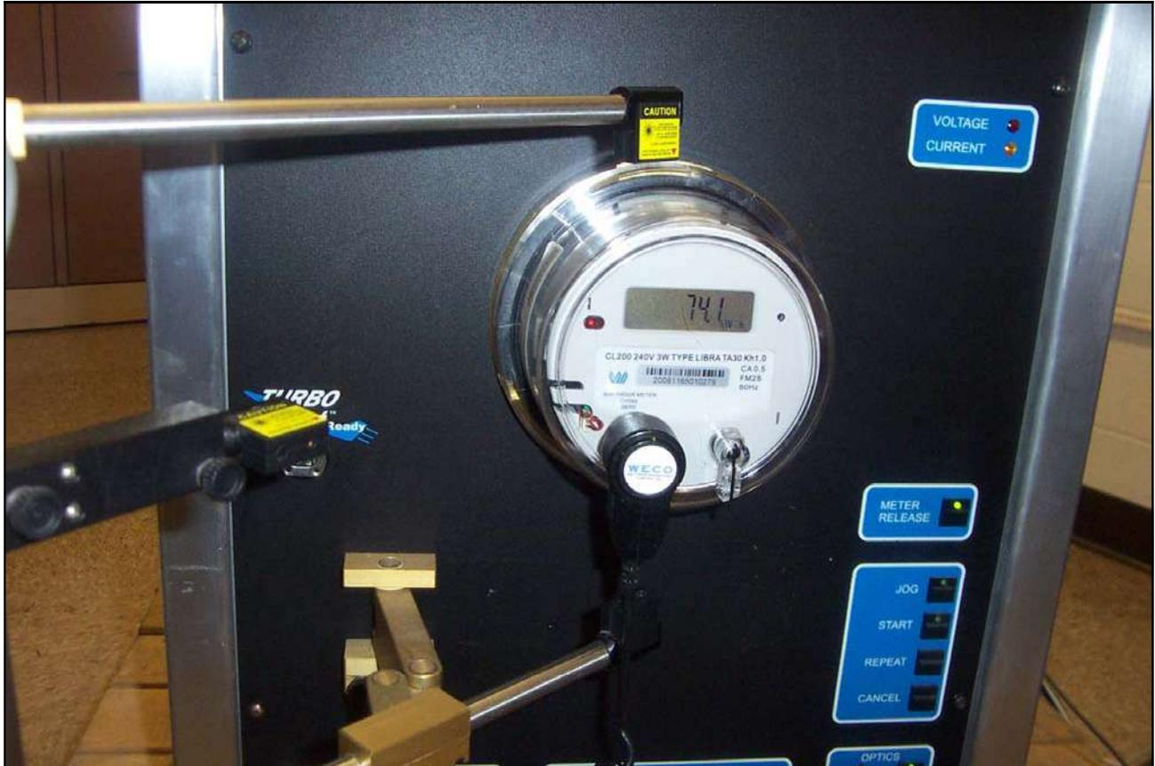
Photograph 46. Test No. 34: Vibration, Performance Verification, Test Setup
