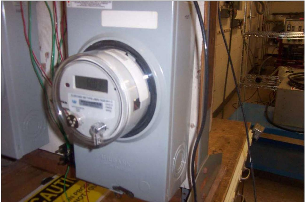
**Photograph 13. Test No. 13: Stability of Performance, Test Setup, Meter Serial No. 10271**
