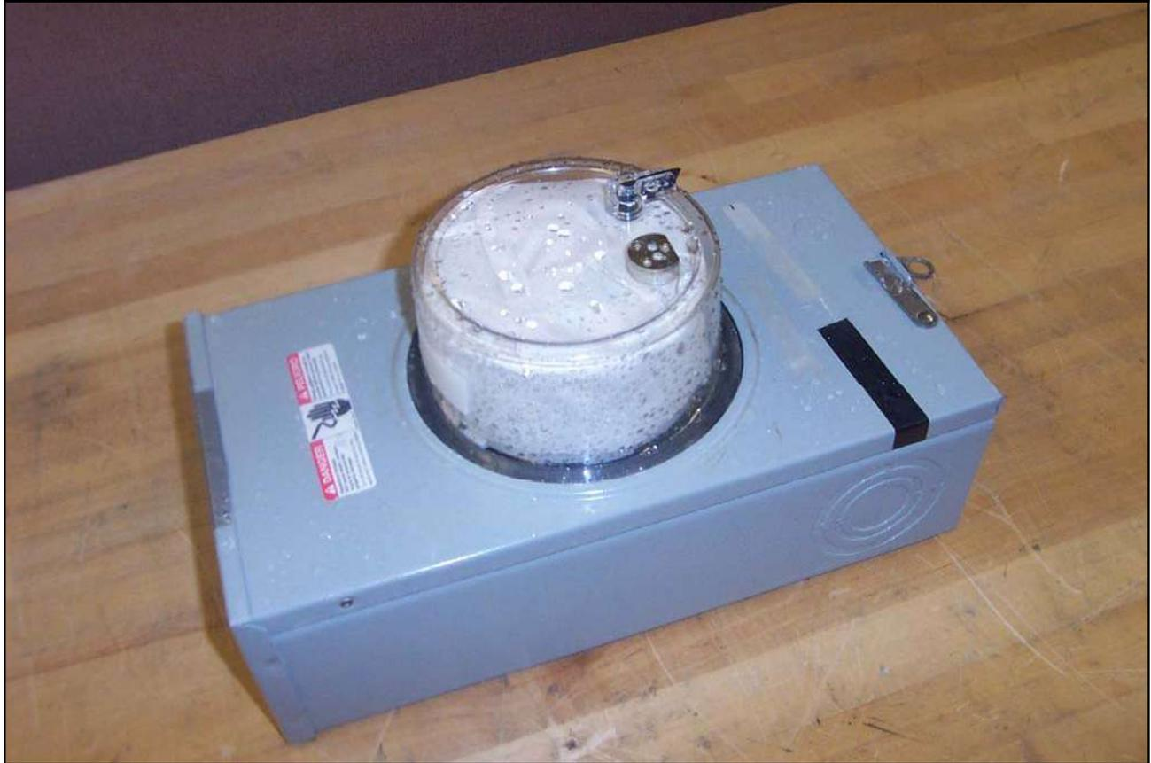
**Photograph 69. Test No. 38: Rain-Tightness, Meter Serial No. 10296, After – 1**
