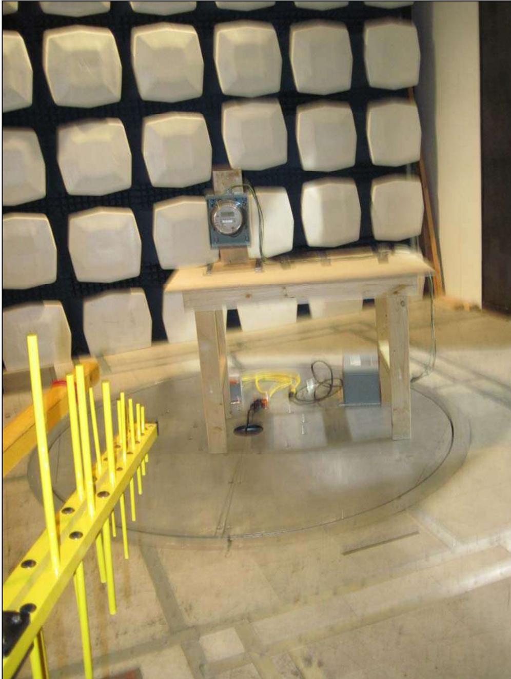
**Photograph 34. Test No. 27: Radio Frequency Radiated Emissions Limits, Retest Setup**
