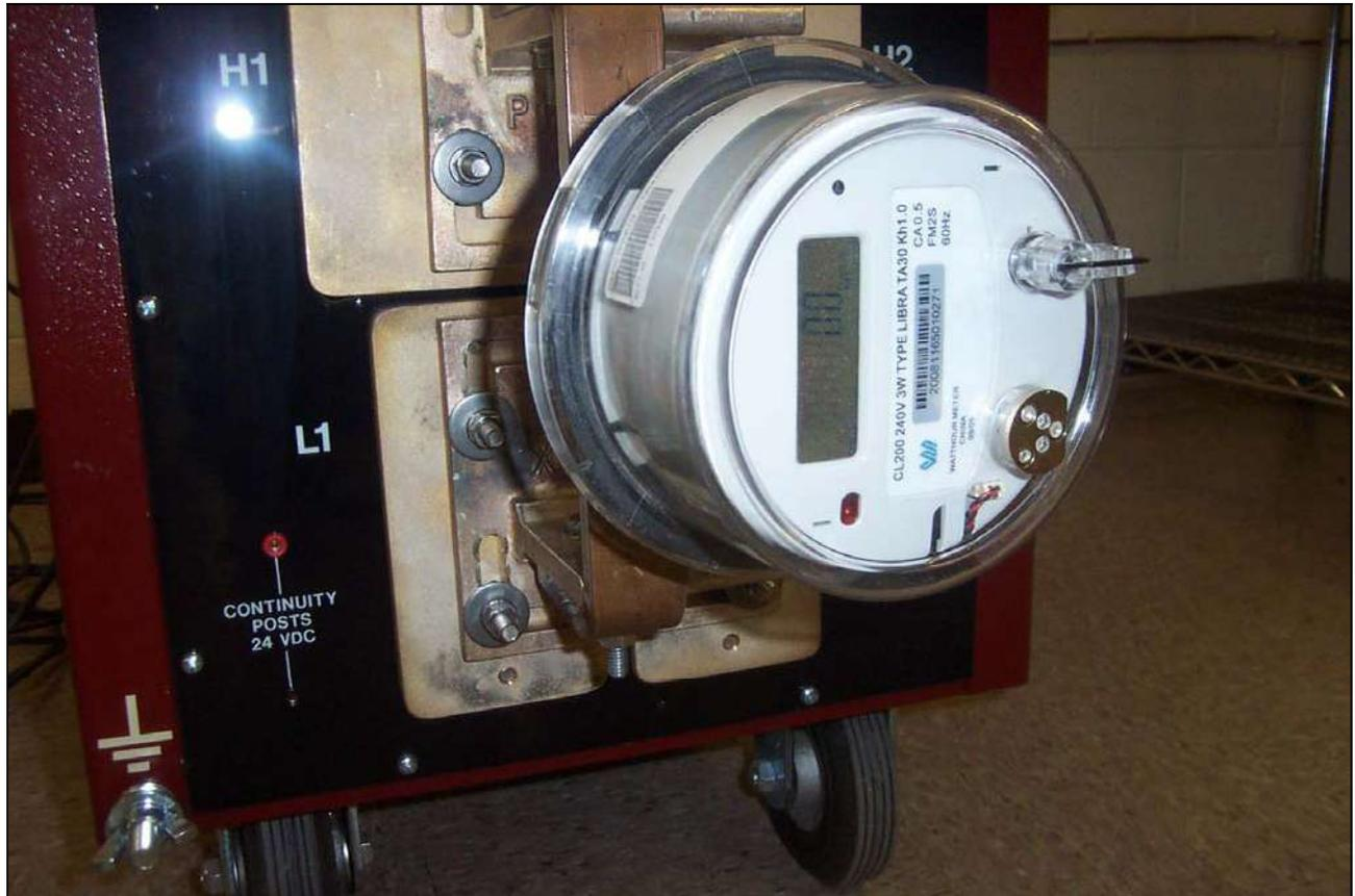
Photograph 26. Test No. 20: Effect of Temporary Overloads, 5.5.3.7.2, 12kA Peak, Overcurrent
