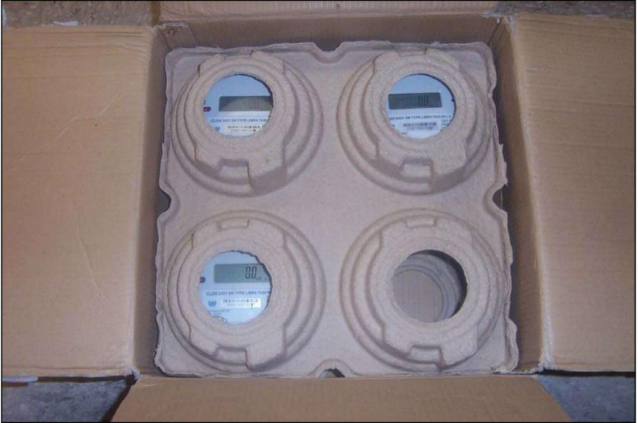
**Photograph 45. Test No. 33: Transportation Drop, After**
