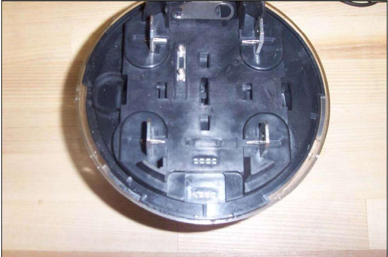
**Photograph 65. Test No. 37: Salt Spray, Meter Serial No. 10297, Rear View**
