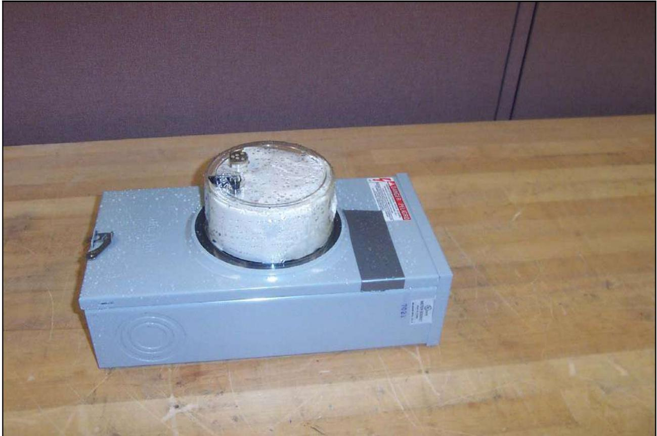
**Photograph 73. Test No. 38: Rain-Tightness, Meter Serial No. 10298, After – 1**
