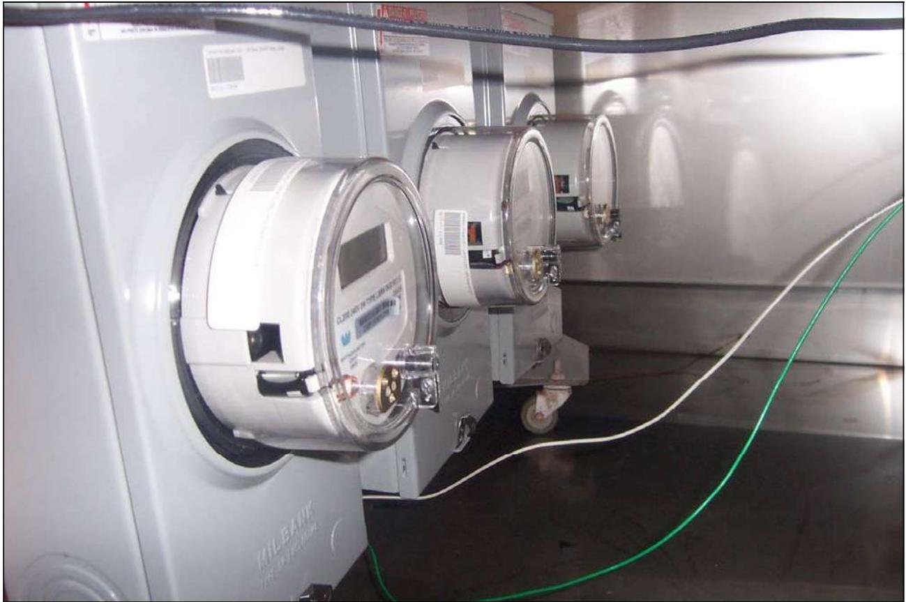
**Photograph 38. Test No. 31: Effects of Variation of Relative Humidity, Test Setup**
