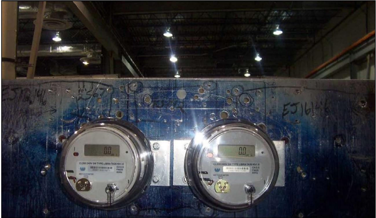
Photograph 49. Test No. 34: Vibration, Y-Axis, Test Setup – 1
