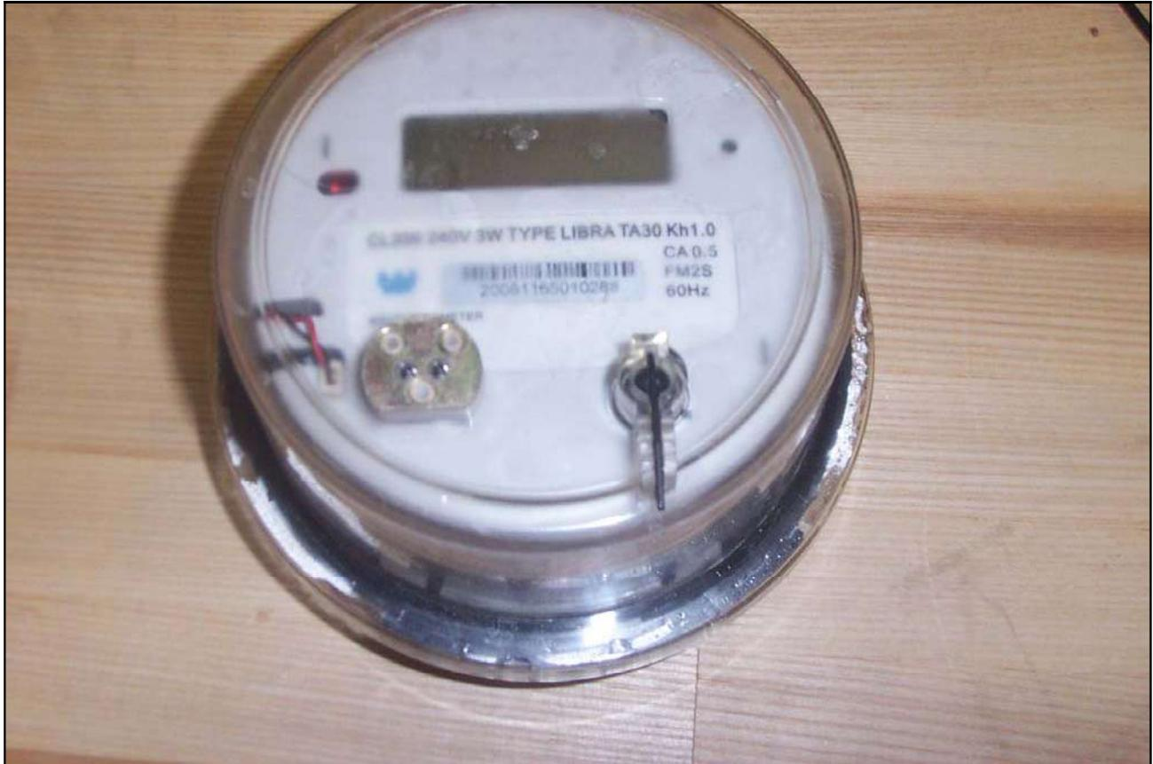
Photograph 66. Test No. 37: Salt Spray, Meter Serial No. 10298, Front View
