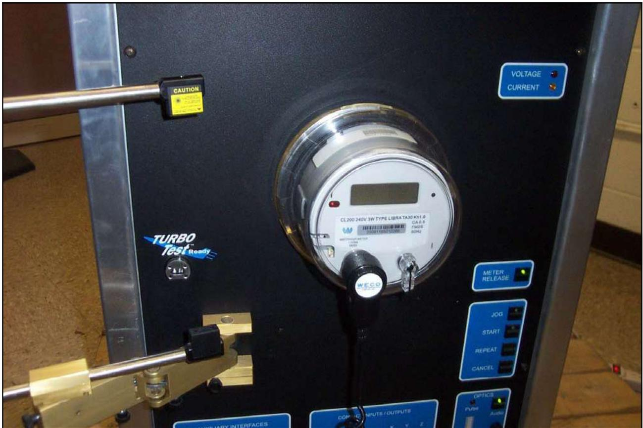
Photograph 8. Test No. 7: Equality of Current Circuits, Test Setup
