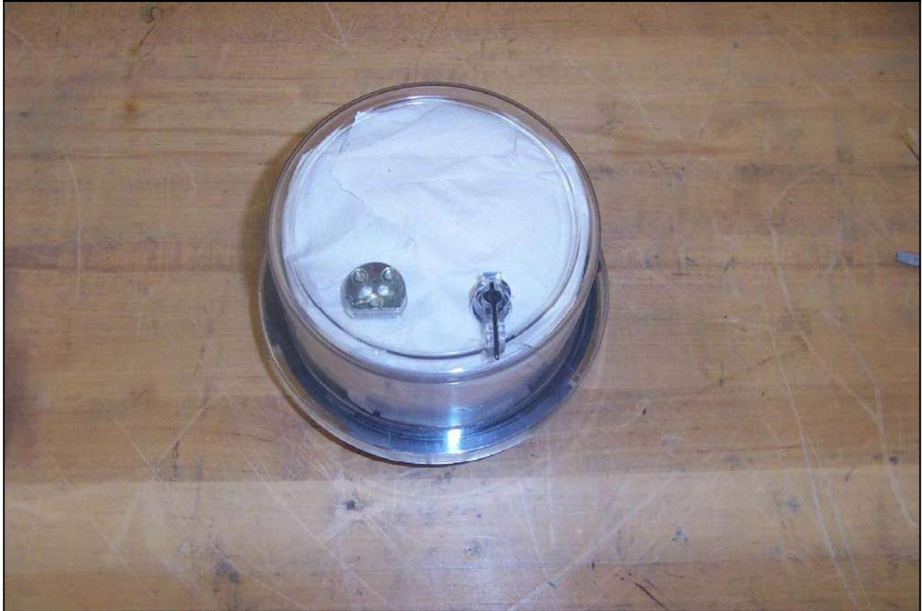
**Photograph 70. Test No. 38: Rain-Tightness, Meter Serial No. 10296, After – 2**
