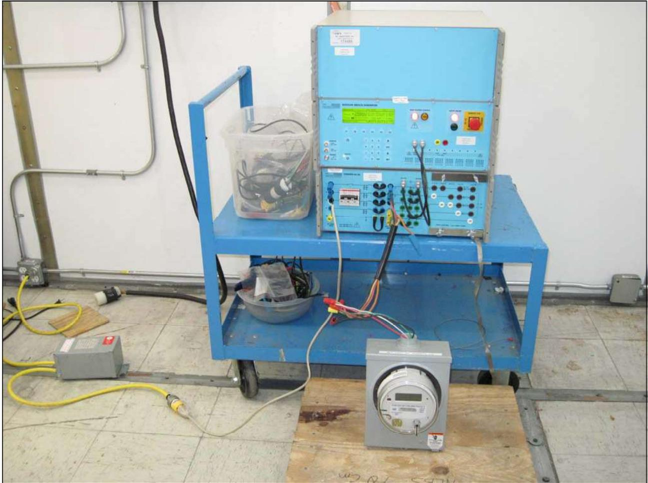
**Photograph 30. Test No. 25a: Oscillatory Surge Withstand Capability, Test Setup**
