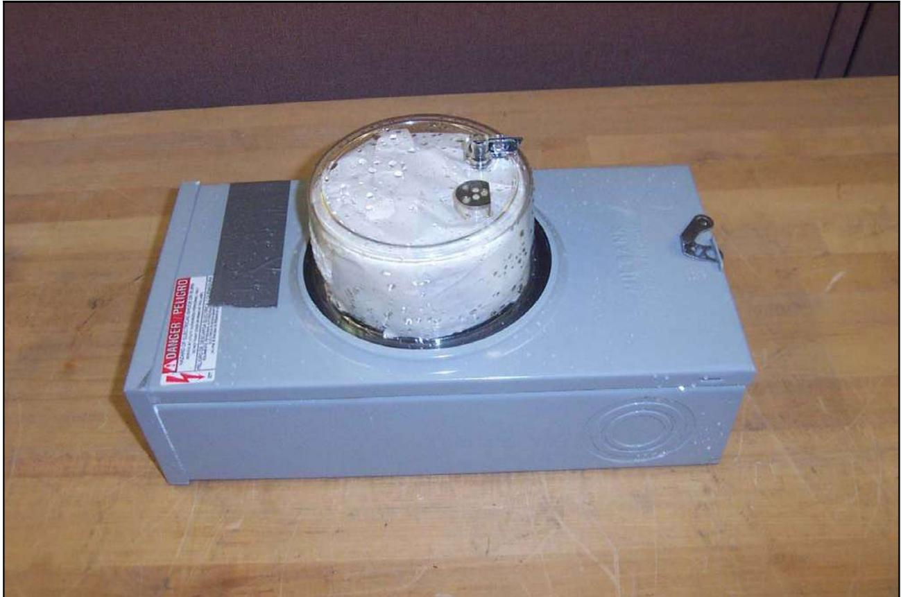
**Photograph 71. Test No. 38: Rain-Tightness, Meter Serial No. 10297, After – 1**
