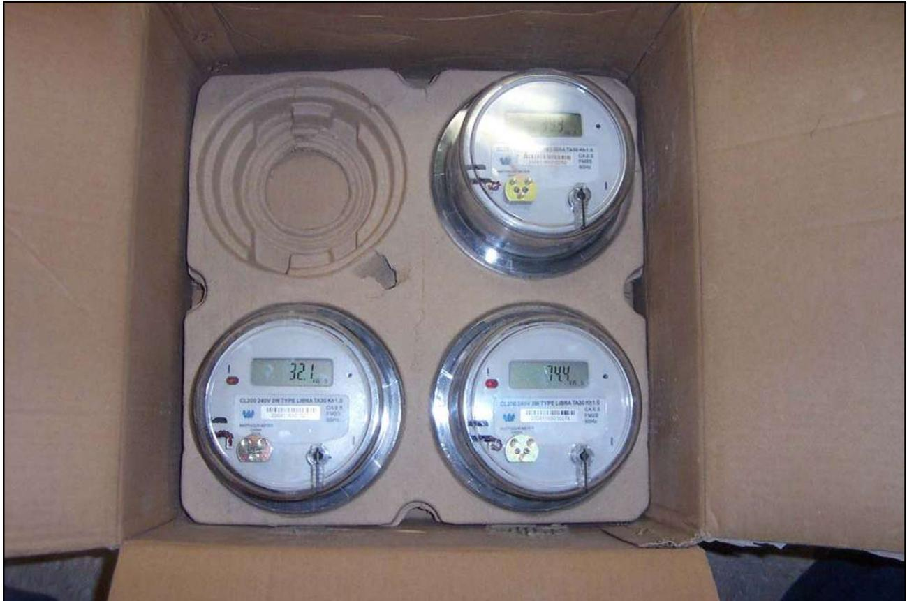
Photograph 55. Test No. 35: Transportation Vibration, After
