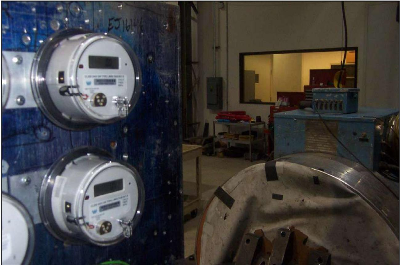
**Photograph 42. Test No. 32: Mechanical Shock, Y-Axis, Test Setup - 2**
