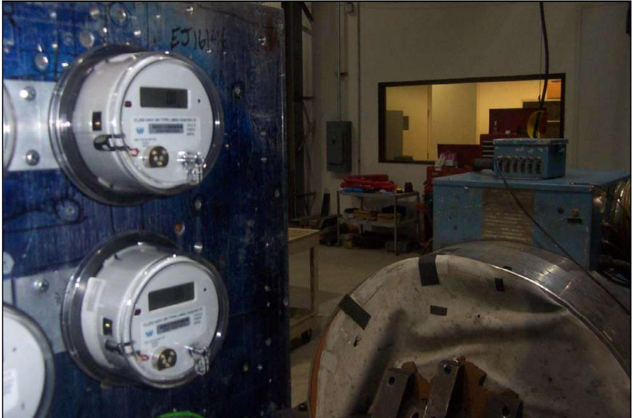
**Photograph 50. Test No. 34: Vibration, Y-Axis, Test Setup – 2**
