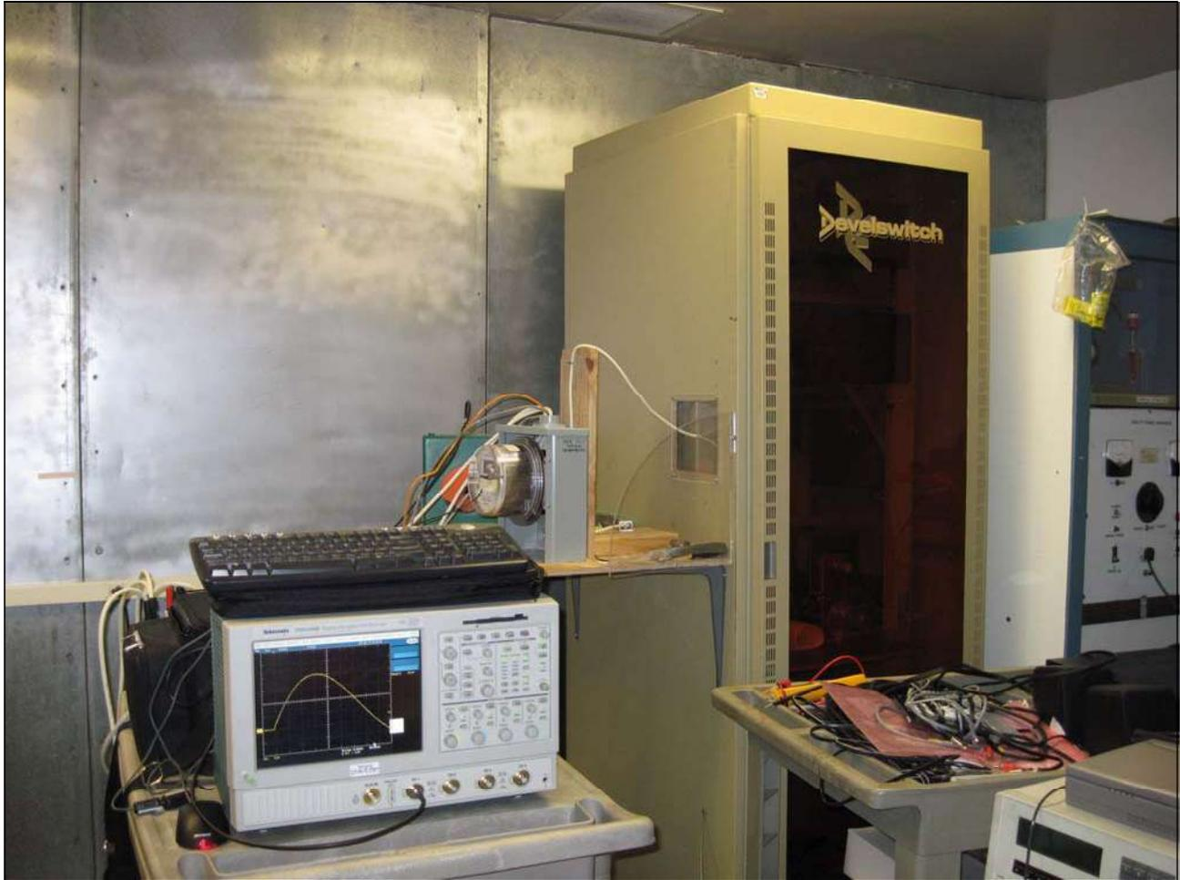
**Photograph 28. Test No. 21: Current Surges in Ground Conductors, Test Setup**
