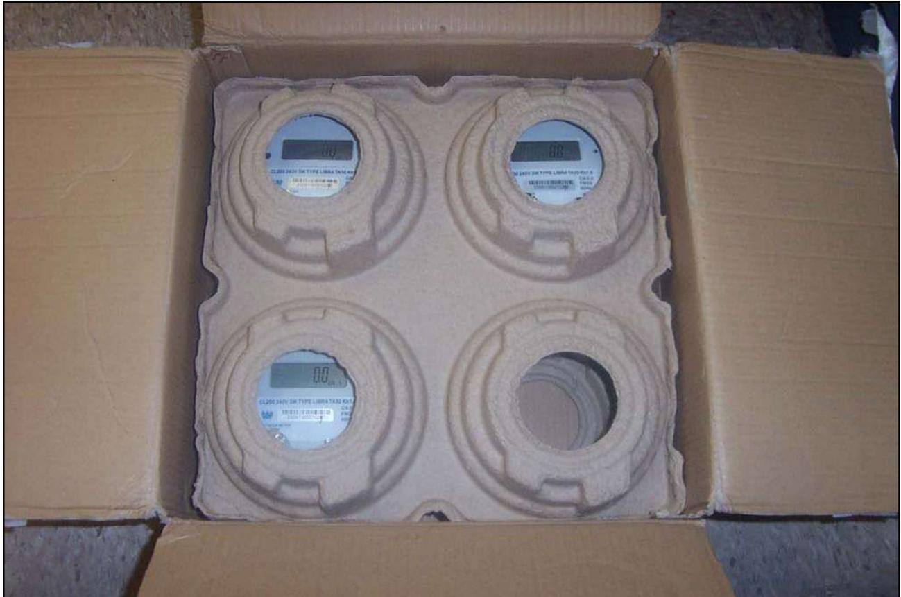
**Photograph 44. Test No. 33: Transportation Drop, Before**
