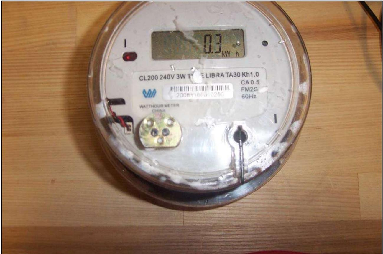
Photograph 62. Test No. 37: Salt Spray, Meter Serial No. 10296, Front View
