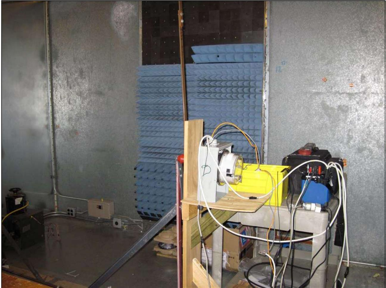
**Photograph 22. Test No. 18: Effect of External Magnetic Field, Test Setup – 2**
