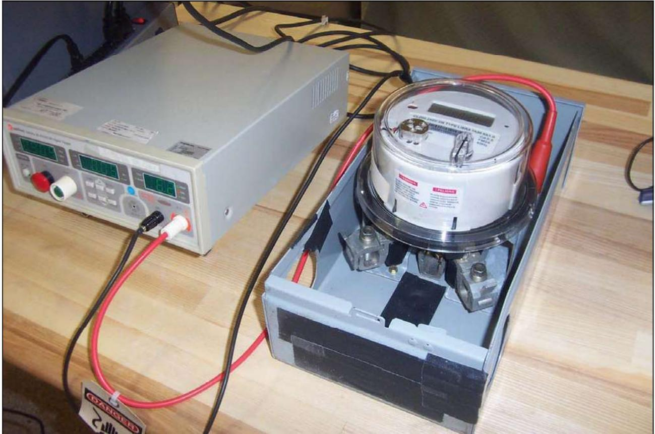
**Photograph 27. Test No. 20: Effect of Temporary Overloads, 5.5.3.7.2, Insulation, Setup**
