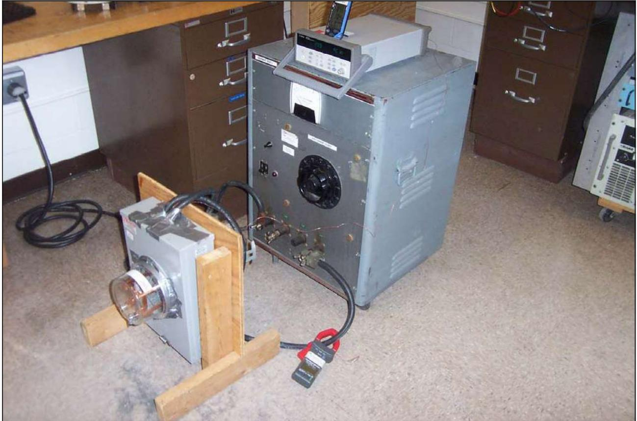
**Photograph 10. Test No. 9: Temperature Rise, Dummy Meter**
