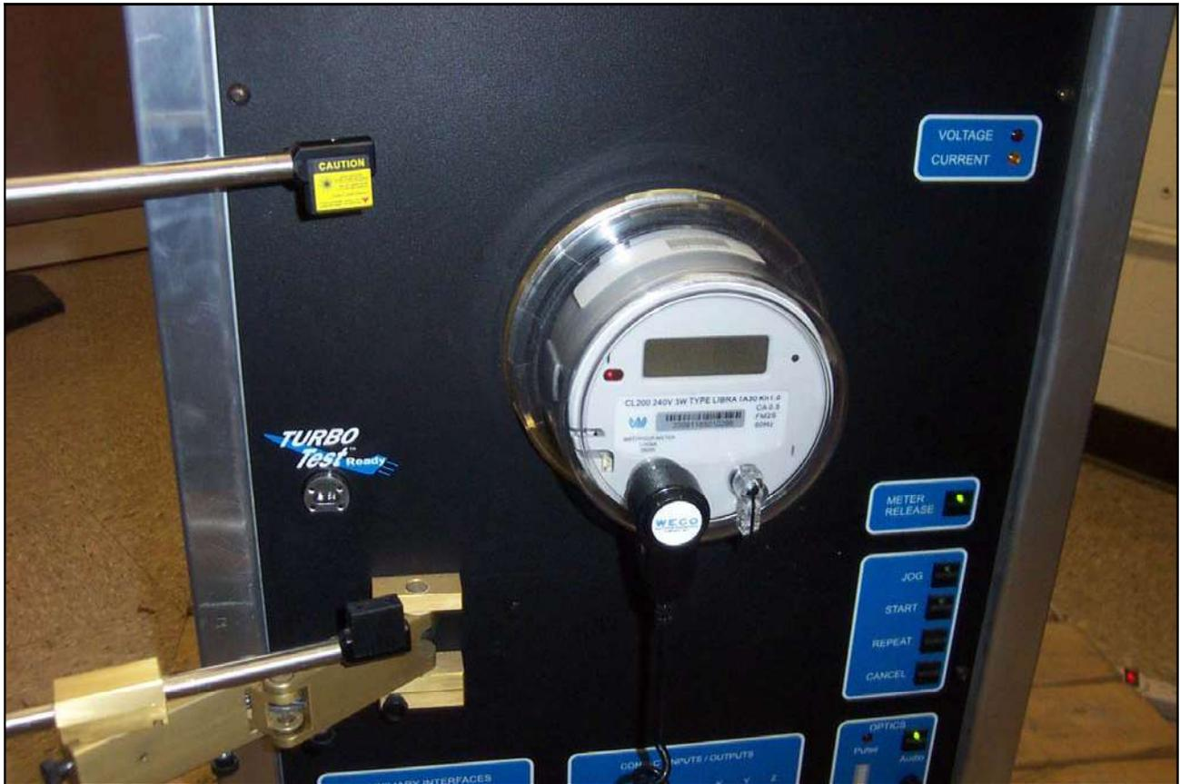
Photograph 5. Test No. 4: Effect of Variation of Power Factor, Test Setup
