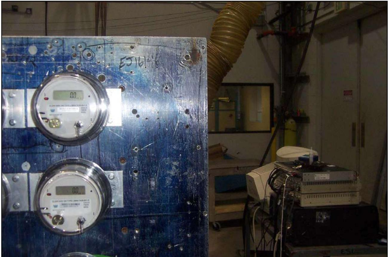
**Photograph 48. Test No. 34: Vibration, X-Axis, Test Setup – 2**
