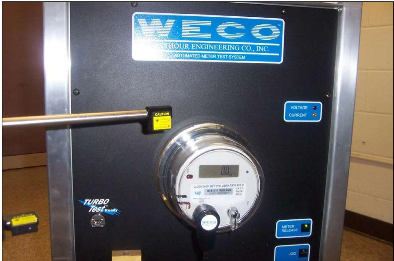
Photograph 12. Test No. 11: Effect of Internal Heating, Test Setup
