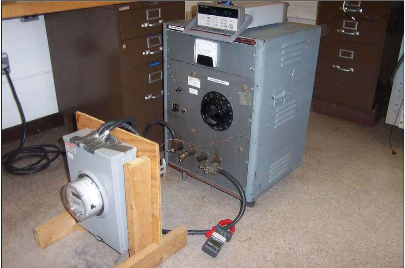
Photograph 11. Test No. 9: Temperature Rise, Test Setup
