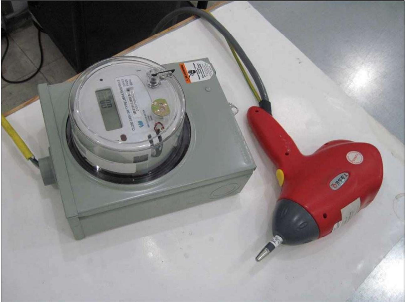
**Photograph 35. Test No. 28: Effect of Electrostatic Discharge (ESD) Test Setup**
