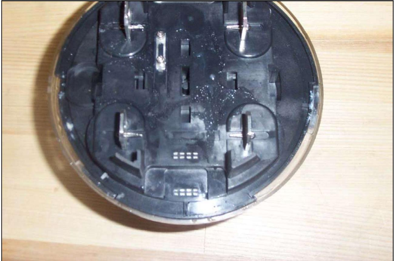
**Photograph 67. Test No. 37: Salt Spray, Meter Serial No. 10298, Rear View**
