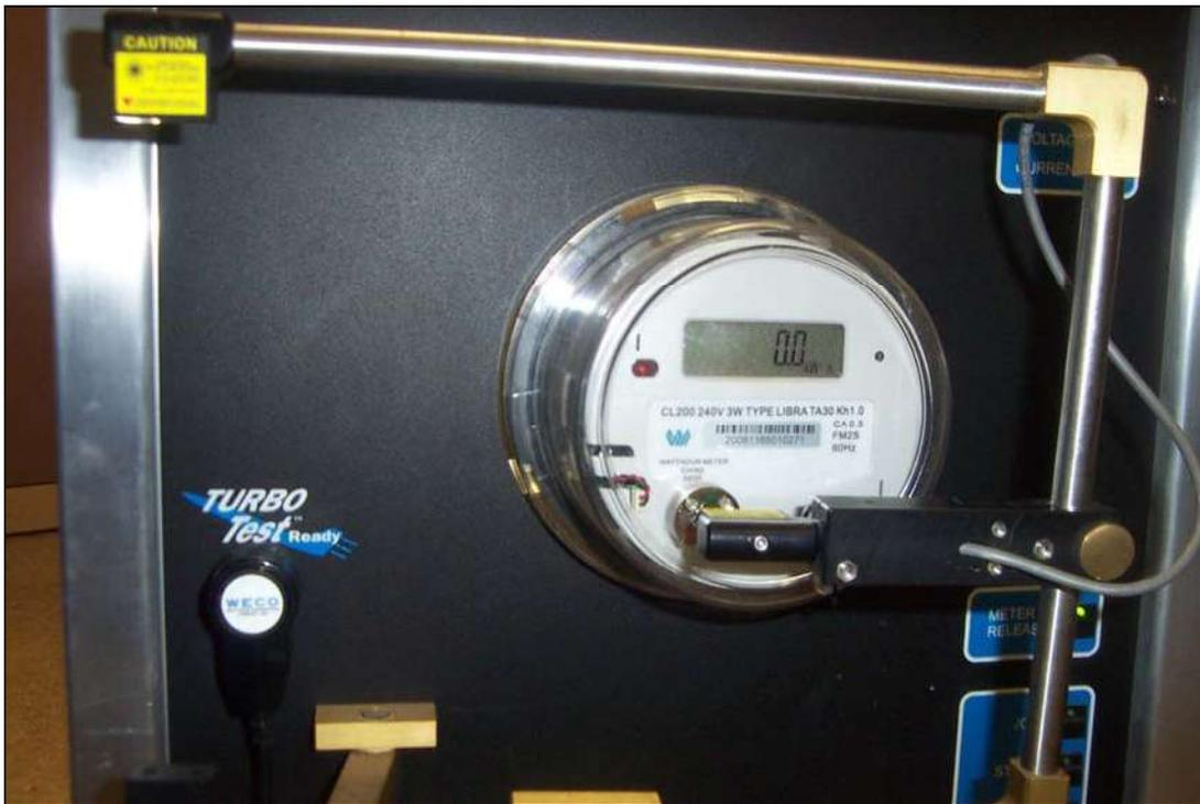
**Photograph 25. Test No. 20: Effect of Temporary Overloads, 5.5.3.7.1, Test Setup**
