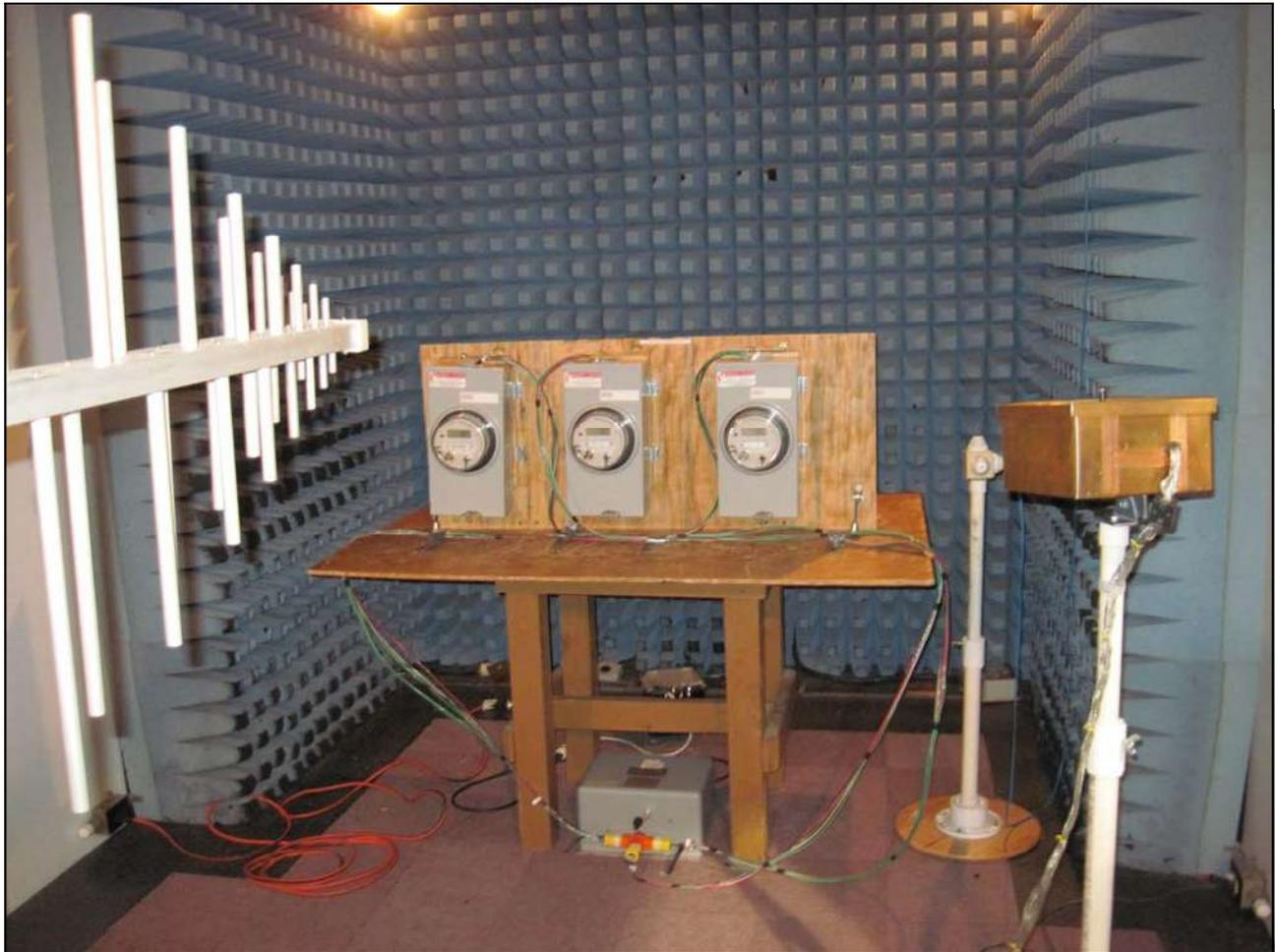
Photograph 31. Test No. 26: Effect of Radio Frequency Interference Test Setup
