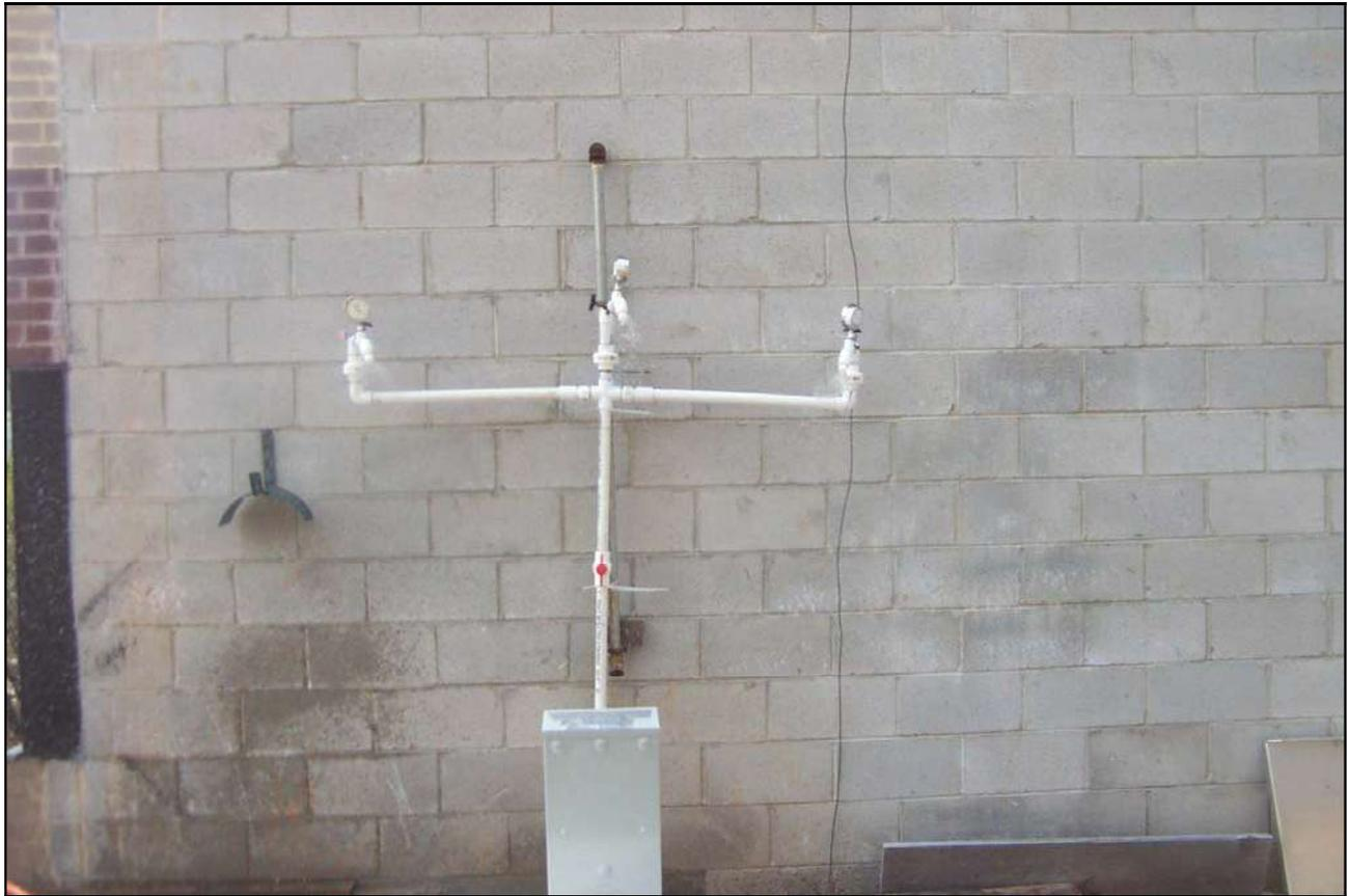
**Photograph 68. Test No. 38: Rain-Tightness, Test Set-up**
