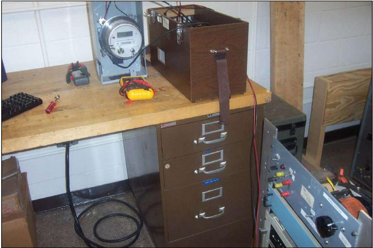
Photograph 9. Test No. 8: Internal Meter Losses, Test Setup
