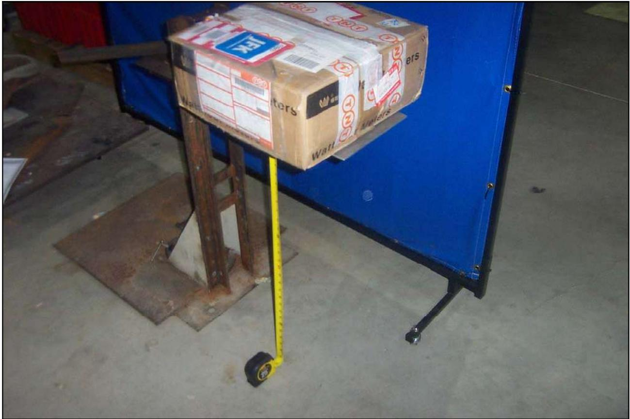
**Photograph 43. Test No. 33: Transportation Drop, Setup**
