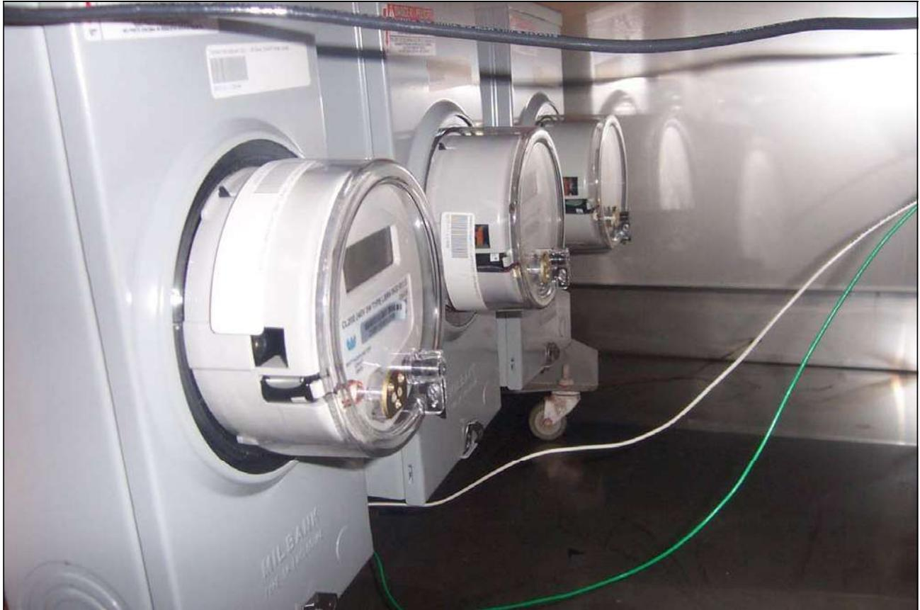
**Photograph 37. Test No. 30: Effects of Variation of Operating Temperature, Test Setup**
