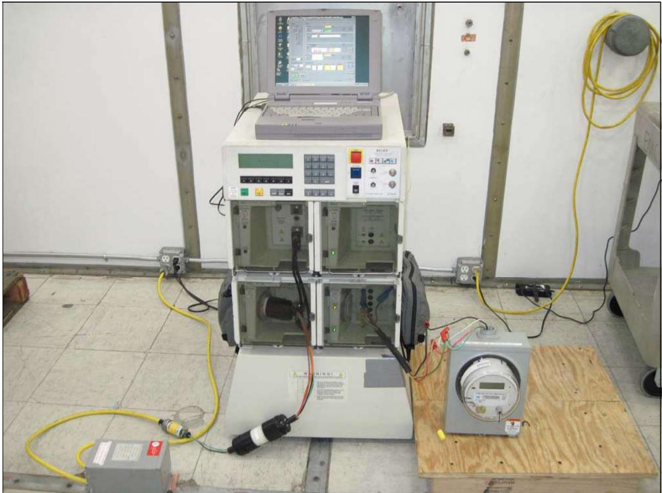
Photograph 19. Test No. 17: Effect of High Voltage Line Surges– 1.2/50  $\mu$ s Combination Wave, Test Setup
