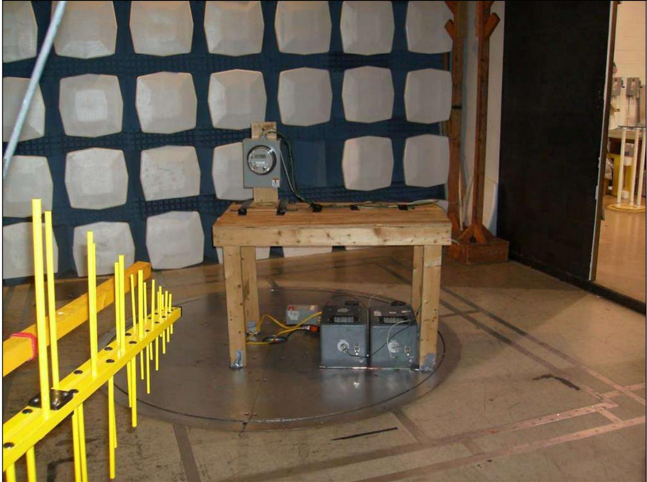
Photograph 33. Test No. 27: Radio Frequency Radiated Emissions Limits Test Setup
