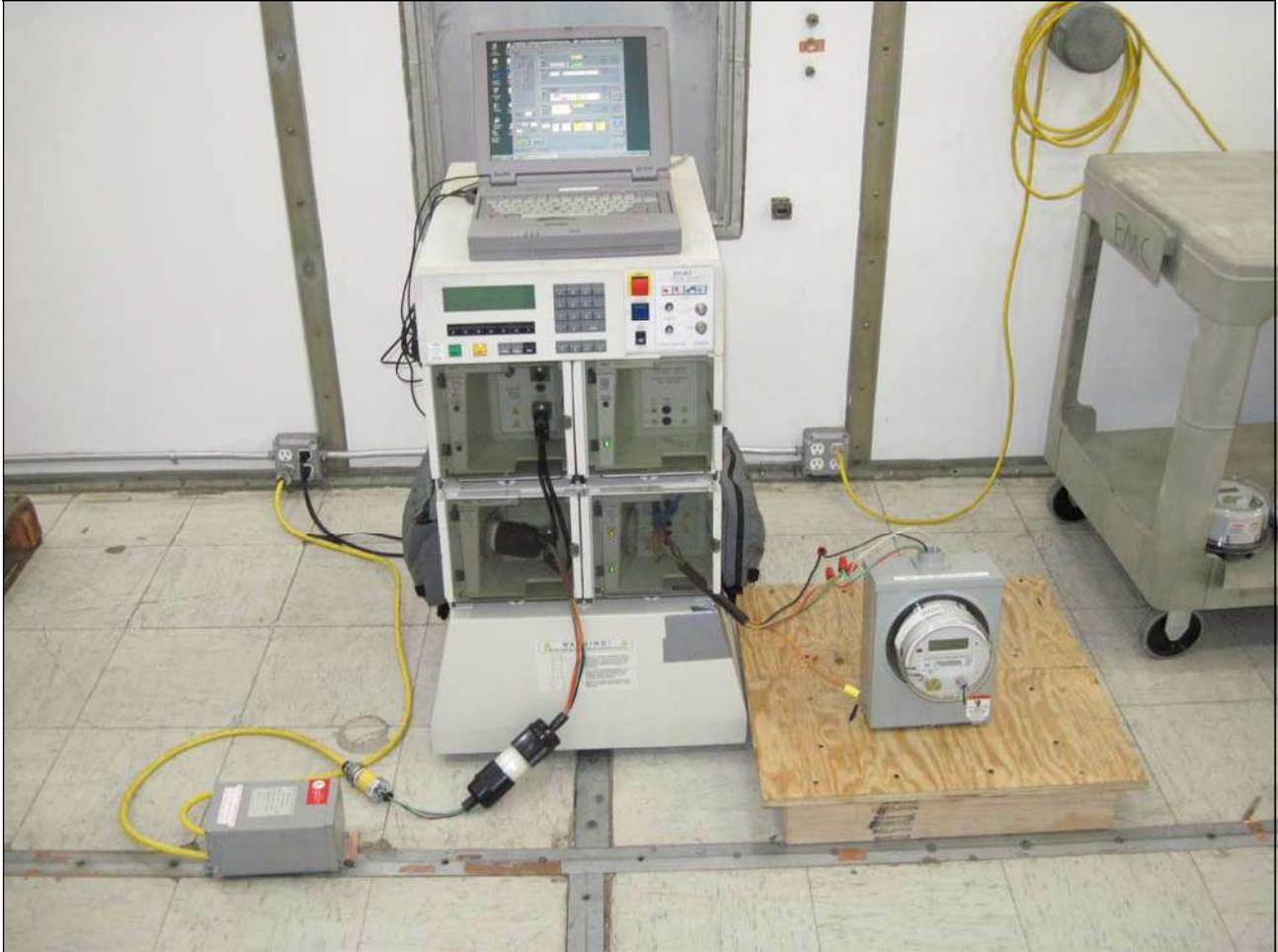
**Photograph 20. Test No. 17: Effect of High Voltage Line Surges– 100 kHz Ring Wave, Test Setup**
