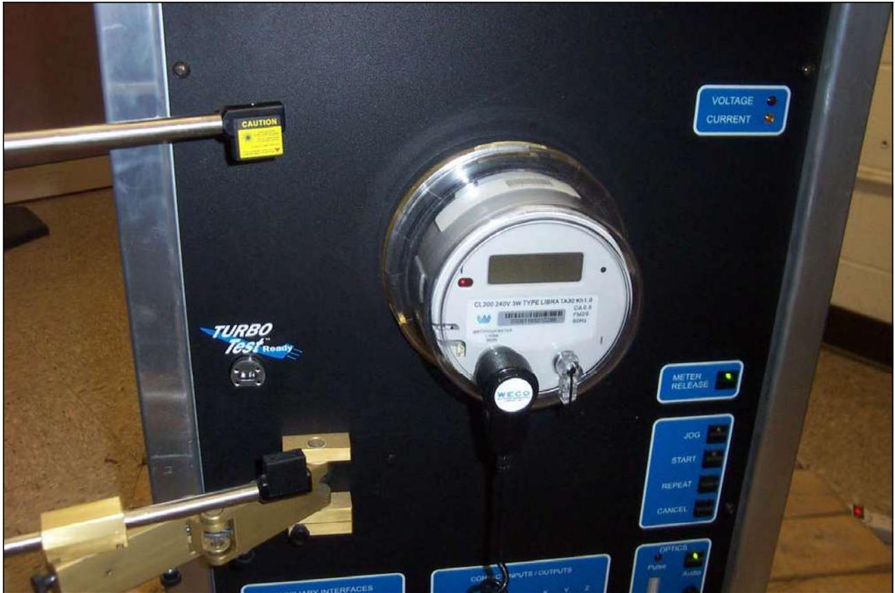
Photograph 3. Test No. 2: Starting Load, Test Setup
